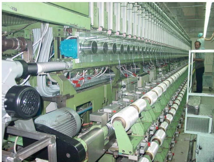
(4: additional heated draw rolls implemented on an existing draw wind machine)
