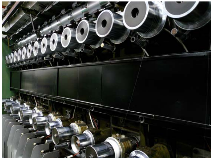
(2: new STS rolls (feed- and draw rolls) on existing bearing housing of an old Rieter draw twist machine)
