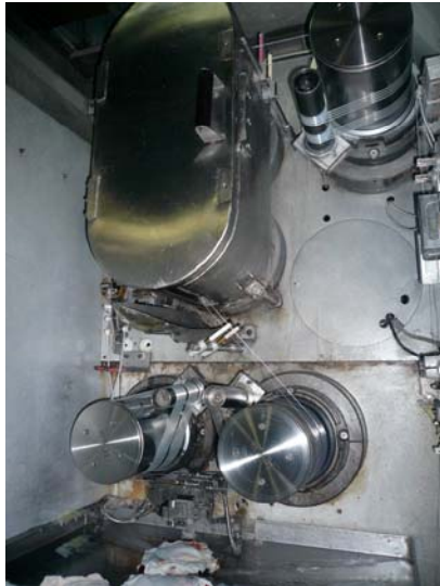
(1: new RTS-rolls in a technical yarn process replacing vapotherm rolls)
